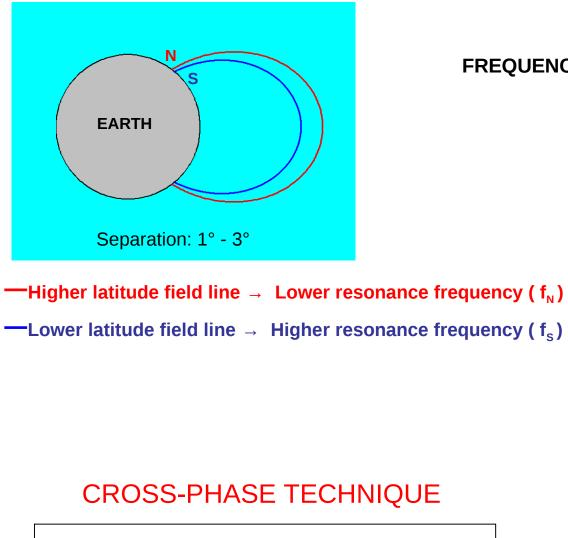
Resonance frequency at the middle point. Identified by a maximum in the phase difference
